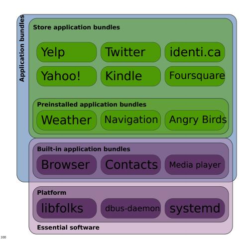
The *platform* is comprised of all the facilities used to boot up the device and perform basic system checks and restorations. It also includes the infrastructural services on which the applications rely, such as the session manager, window manager, message bus and configuration storage service, and the software libraries shared between components.
